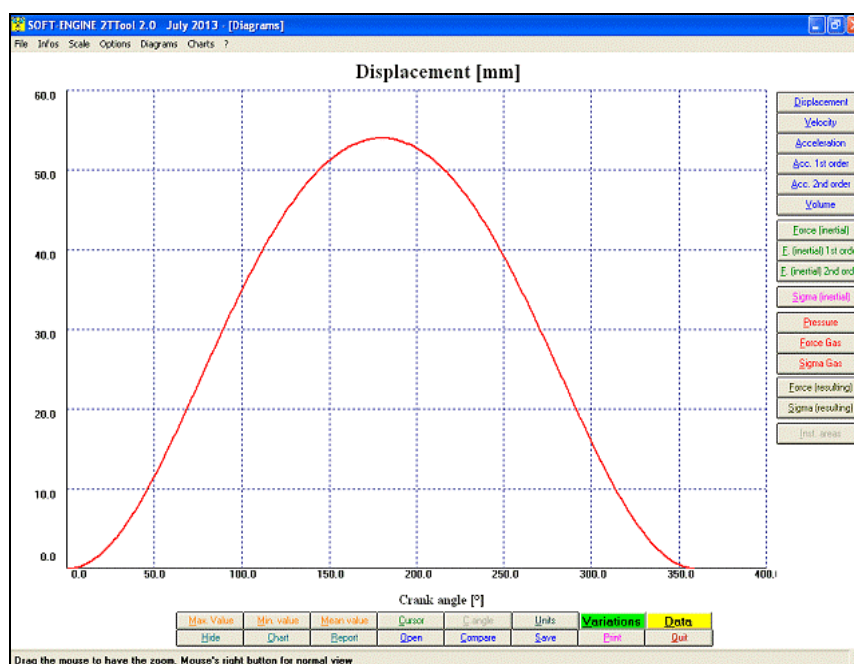
Crankshaft (kinematic) - piston Displacement diagram
