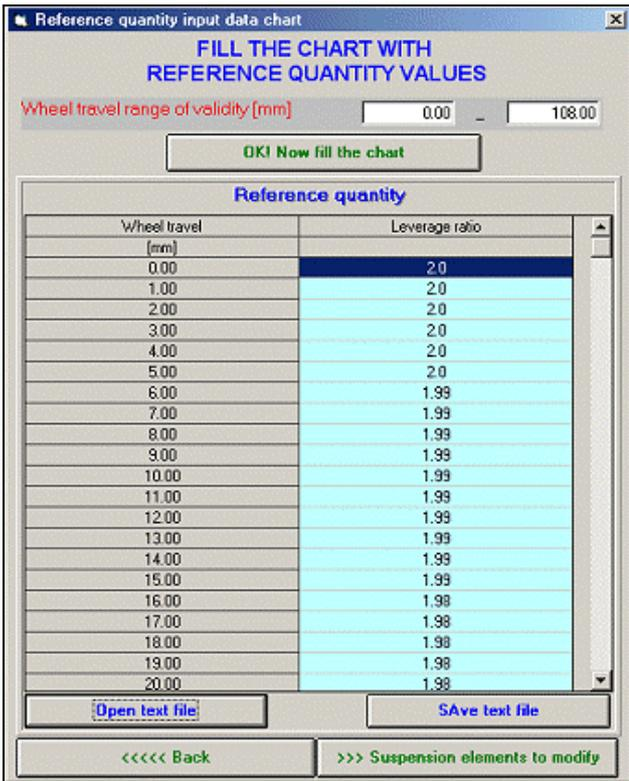
Reverse function procedure: it is possible to import experimental data from text files for references.
