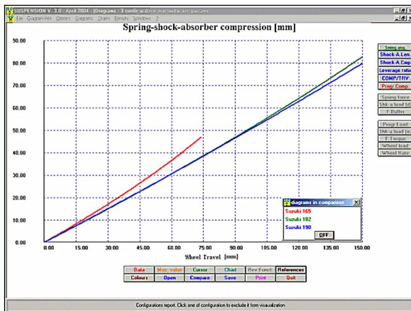
Suzuki GSX-R 1000 2004. "Shock absorber compression" comparison diagram
