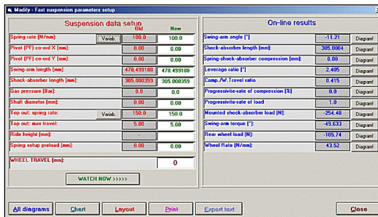
*Fast layout set-up procedure: itis a very quick method to modify suspension main factors*
