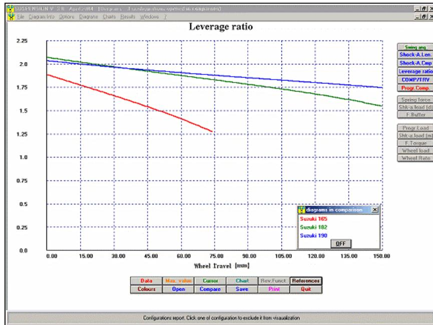
Suzuki GSX-R 1000 2004. "Leverage ratio" comparison diagram
