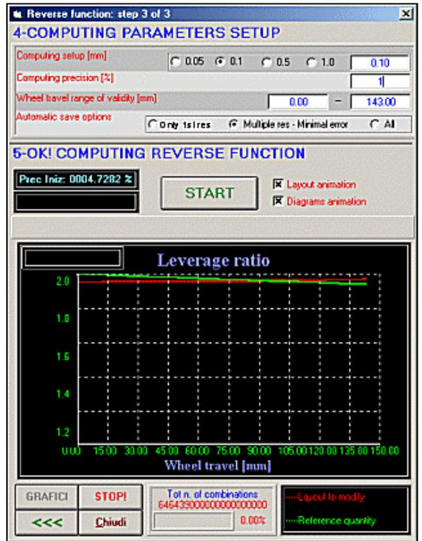
Reverse Function procedure: automatic computation. It is possible to see how red leverage ratio modifies until it is equal to green one.
