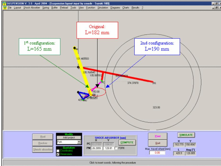
Suzuki GSX-R 1000 2004. Original Rod's length is 182.00 mm
