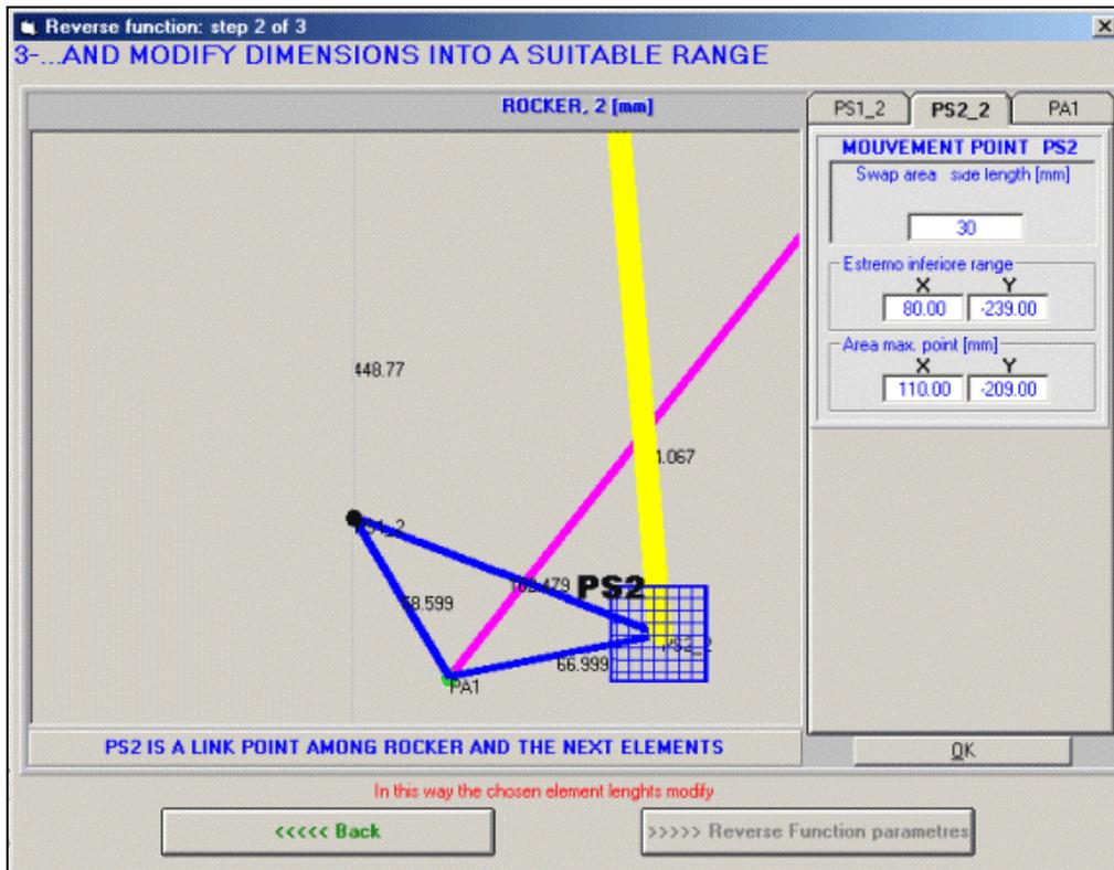
Reverse Function procedure: swapping areas PS2 vertex data input. It is possible to define a swapping area for each vertex. "Swapping area" is the space area in which selected vertexes must move during Reverse Function procedure
